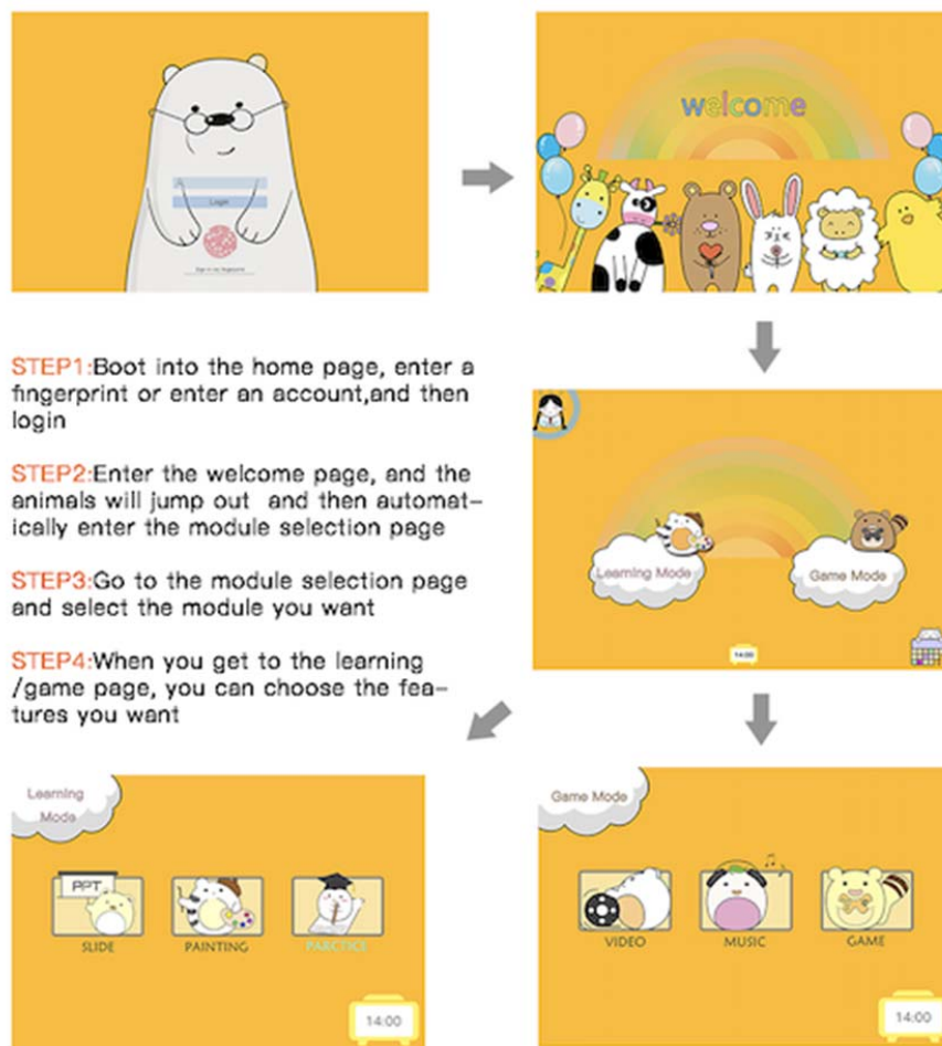
Fig. 10 Eks(x), touch-screen and main interface design
